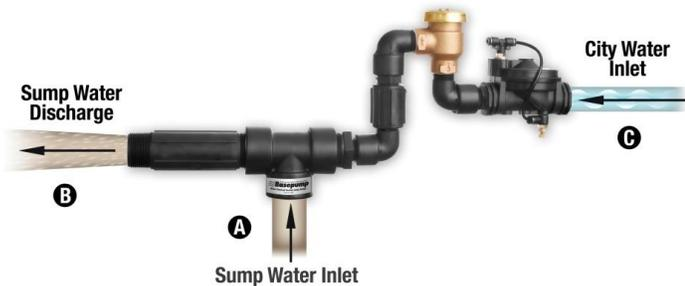
The Basepump with the AVB optional backflow preventer adds an additional level of protection. When a backflow condition occurs, The AVB valve allows air to enter the system, which breaks any siphon effect.
