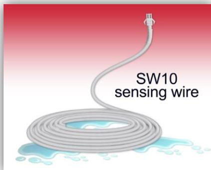
The **#SW10** is an absorbent water sensing wire consisting of two twisted metallic wires isolated from each other by a polypropylene insulator and surrounded by a white polyethylene mesh braided jacket. The sensing wires are end terminated with a male and female snap connector. Sensing wires **#SW10** may be snap connected in series to a maximum of 50 feet
